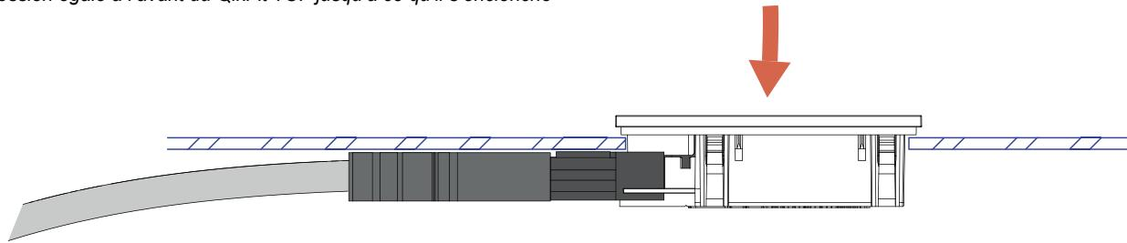
Alternatively, if rear access is available QikFit TUF can be fitted into the panel first (as above), and then the GST18i3 cable attached afterwards.
