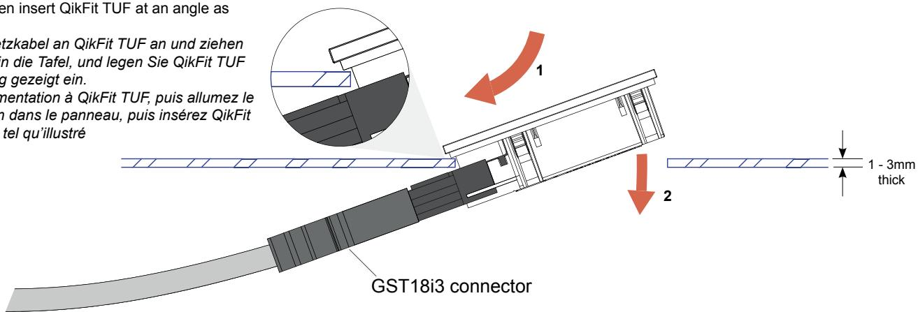
2. Apply equal pressure across the front of the QikFit TUF until it clicks into place
